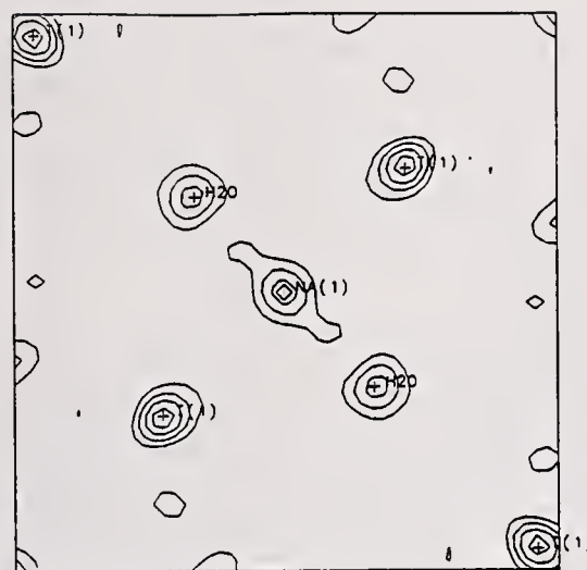
Figure 2. Difference-Fourier map of analcime at z=0 , calculated without Na or \text{H}_2\text{O} in the model. Contours are drawn at 2.0, 4.0, 6.0, and 8.0 electrons.
